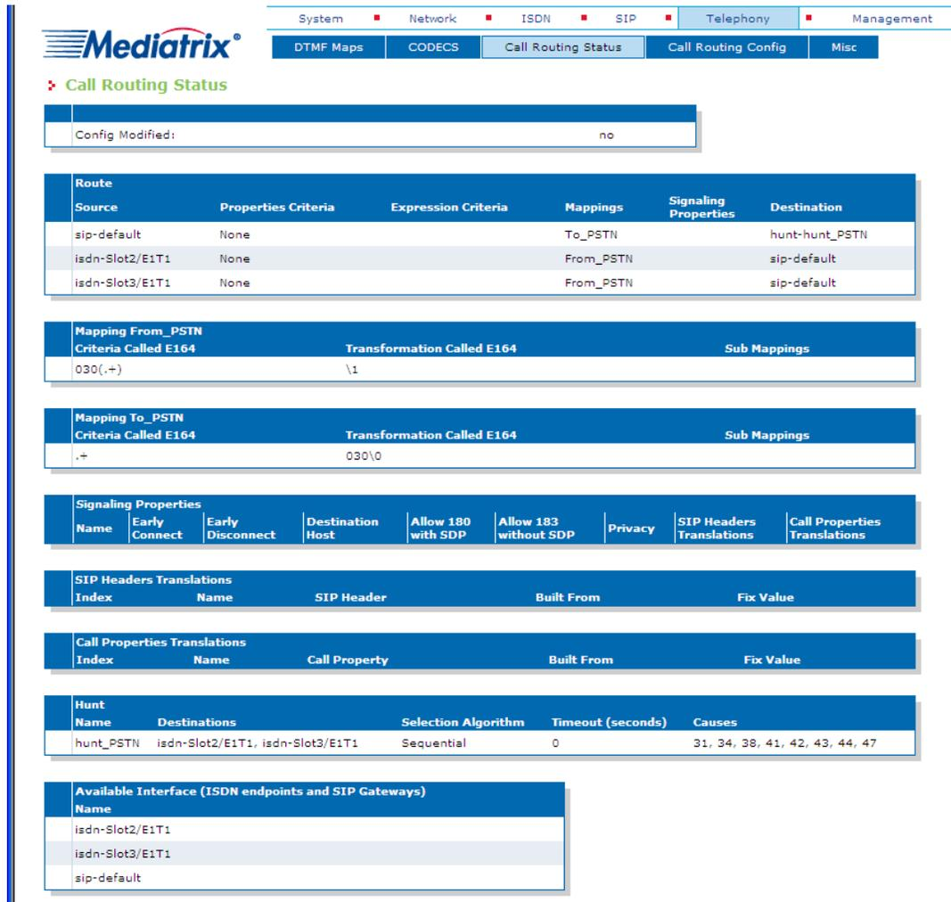
The screenshot shows the Mediatrix web interface for 'Call Routing Status'. It includes a navigation bar with tabs for System, Network, ISDN, SIP, Telephony, and Management. Under the Telephony tab, there are sub-tabs for DTMF Maps, CODECS, Call Routing Status, Call Routing Config, and Misc. The main content area displays several configuration sections:
