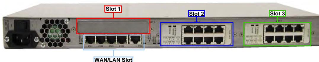
[Figure 3](#) shows the rear panel of the Mediatrix 3300.
