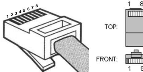
When connecting an Ethernet cable to the Mediatrix 4104, use a standard telecommunication cord with a minimum of 26 AWG wire size. It is possible to use either a crossover or straight Ethernet cable to connect in the Ethernet connectors. These connectors perform automatic MDI / MDIX detection, meaning that they adapt to the type of cable connected to them.
